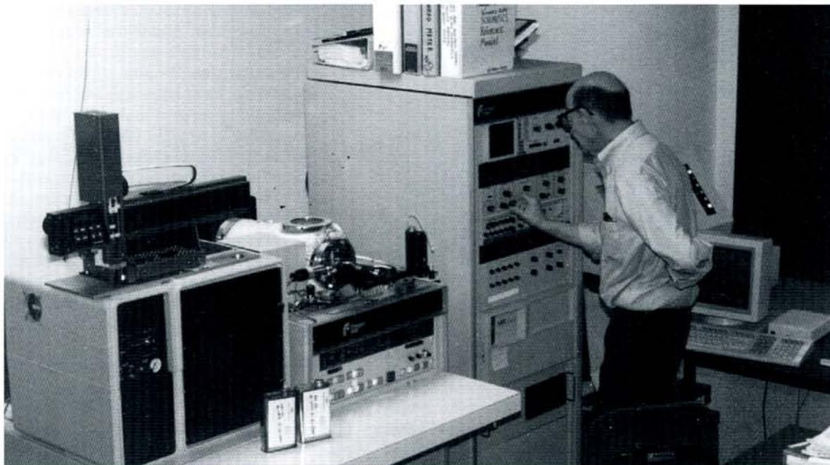
Fig. 3. Combination GC and MS first separates samples by boiling range, then determines molecular weights and saturations.
